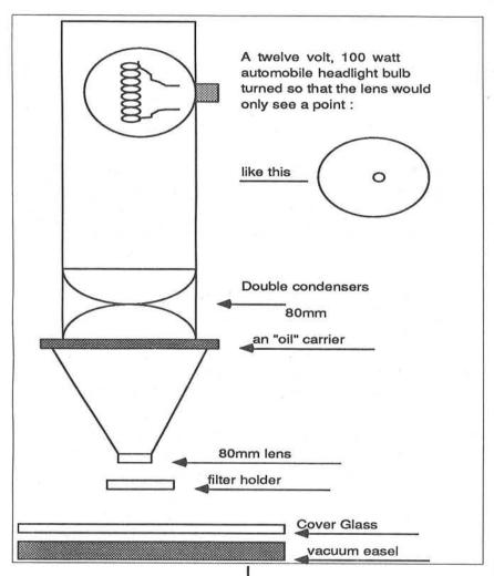
the same refraction index as glass and were able to see their objects much more clearly. It just so happened, that castor oil had a very close refraction index to the glass we were using.
