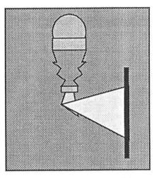
The only thing wrong with this method is, that you will have to construct a wall mounted vacuum carrier, and if you have to remove masks in order to replace them with different masks, the entire assembly must be as rigid as a rock.
