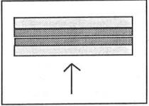
However, if you try to make a print with this combination, and want the image to read correctly, you will have to expose through the mask. This is not a good idea. But, when you are ready to make your print, use a front surface mirror to project the image to the wall and project the image through the base of the transparency. The mirror will turn the image around so that it reads right.
