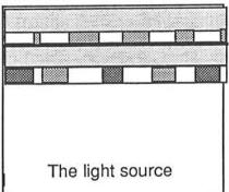
and place it into the enlarger carrier, a normal 150mm lens will give you a better chance of making a clean print with no register lines showing. However, if you use a shorter focal length lens such as a 135mm, you will experience these unwanted lines.
