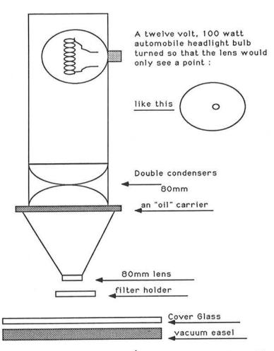
The bulb was a simple 12 volt automobile bulb. The filament was turned in such a way so that the lens could only see the end of the filament and not its entire length. This worked fine, except for the dirt and scratches.
