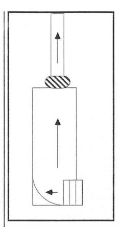
A simple dryer like the illustration above is all that is necessary for drying the delicate gelatin pigment images. Warm air produced by a simple room heater, and a small blower at the top of the unit to remove the air from the box.
