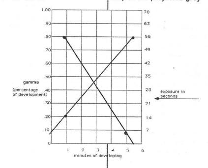
In order to use the chart properly, find the required gamma on the left side of the chart, look to the right until it intersects the developing line, then look down to the bottom of the chart to find the time of development. Then, while on the development time, look up until you interect the exposure line, then look to the right to find the correct exposure. You must do this procedure for the other two filters as
