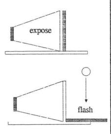
This flashing action will add density to the lower portions of the scale and produce less contrast.
