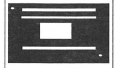
This represents the copy negative shot using litho film. Notice the pin holes used in registration.
