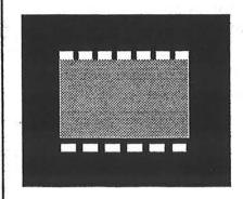
The three step grey scale is used by placing it on the bottom side of the glass before the masks are exposed. This eliminates any problems with the thickness of the film being an obstruction.
