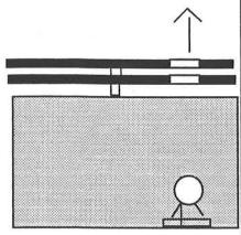
By building a simple wooden box with a standard light bulb fixture screwed into the bottom and a #213 enlarging bulb screwed into it. Two circular sheets of wood or sheet metal with filters on one of them and Waterhouse F stops cut out of it will enable you to make accurate and repeatable exposures without any color
