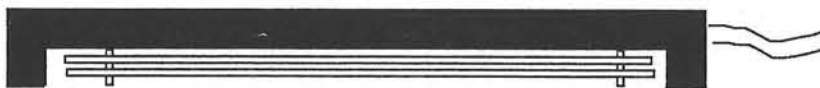
An upside vacuum carrier that allows the elimination of the bottom glass
